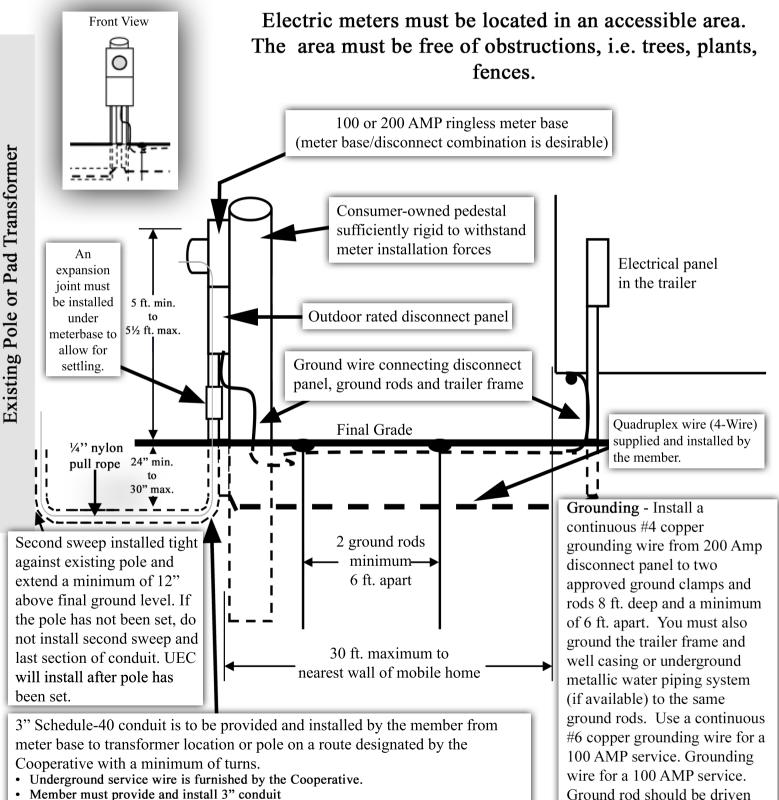
• Member must provide and install 3" conduit
