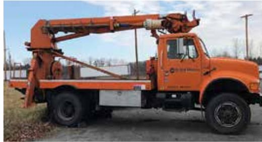
**1989 International 4800, 4 x 4, 150,612 miles, DT 466 diesel engine – 210 H.P., Spicer S-90 9000lb front-drive axle, Fabco TC-38, 2-speed transfer case, Spicer 5-speed transmission, International N-175, 17,500lb rear axle, Altec digger derrick, model D-820 BC, 3-stage corner-mount derrick-no auger, Rope tip winch, Rear winch – Braden PD-18 hydraulic, flat bed, engine overhaul – 10,000 miles ago.**
